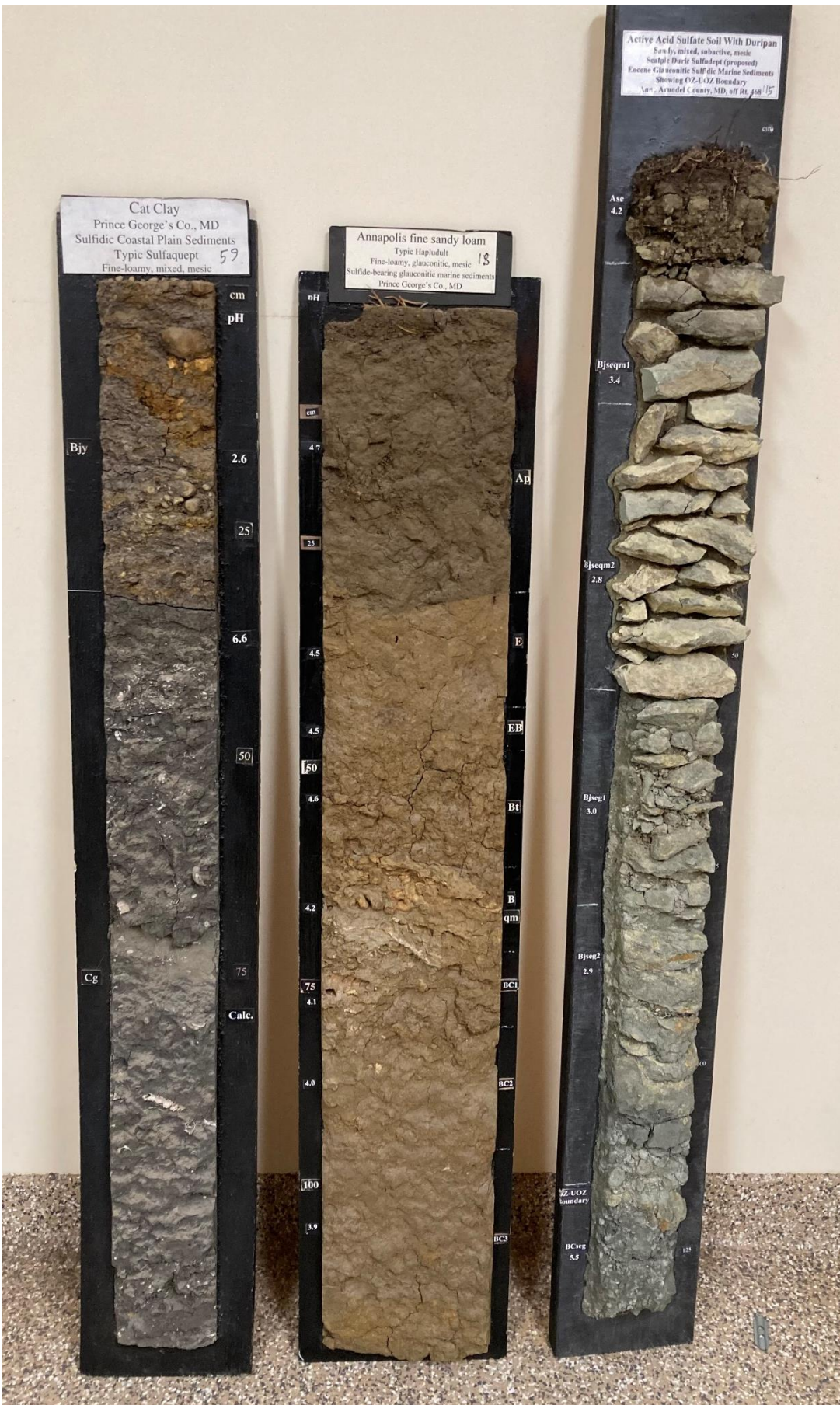
Fig. 1. Photo of 3 monoliths featured in this article, each described and presented in more detail in subsequent pages. Collection monolith No. 18, of a post-active acid sulfate soil, Annapolis fine sandy loam, from a cultivated field, note the thick Ap horizon, is in the center. Collection monolith 59, labeled Cat Clay, of an active acid sulfate soil collected from a scalped land surface within a cloverleaf of the Washington, DC beltway is on the left. On the right, is another active acid sulfate soil, monolith No. 115, from a roadcut on Rt. 426 in Anne Arundel County. It has silica-cemented horizons, still containing sulfide minerals at its surface that helps explain the genesis of a zone with silica cemented casts of shells in the Annapolis monolith.
