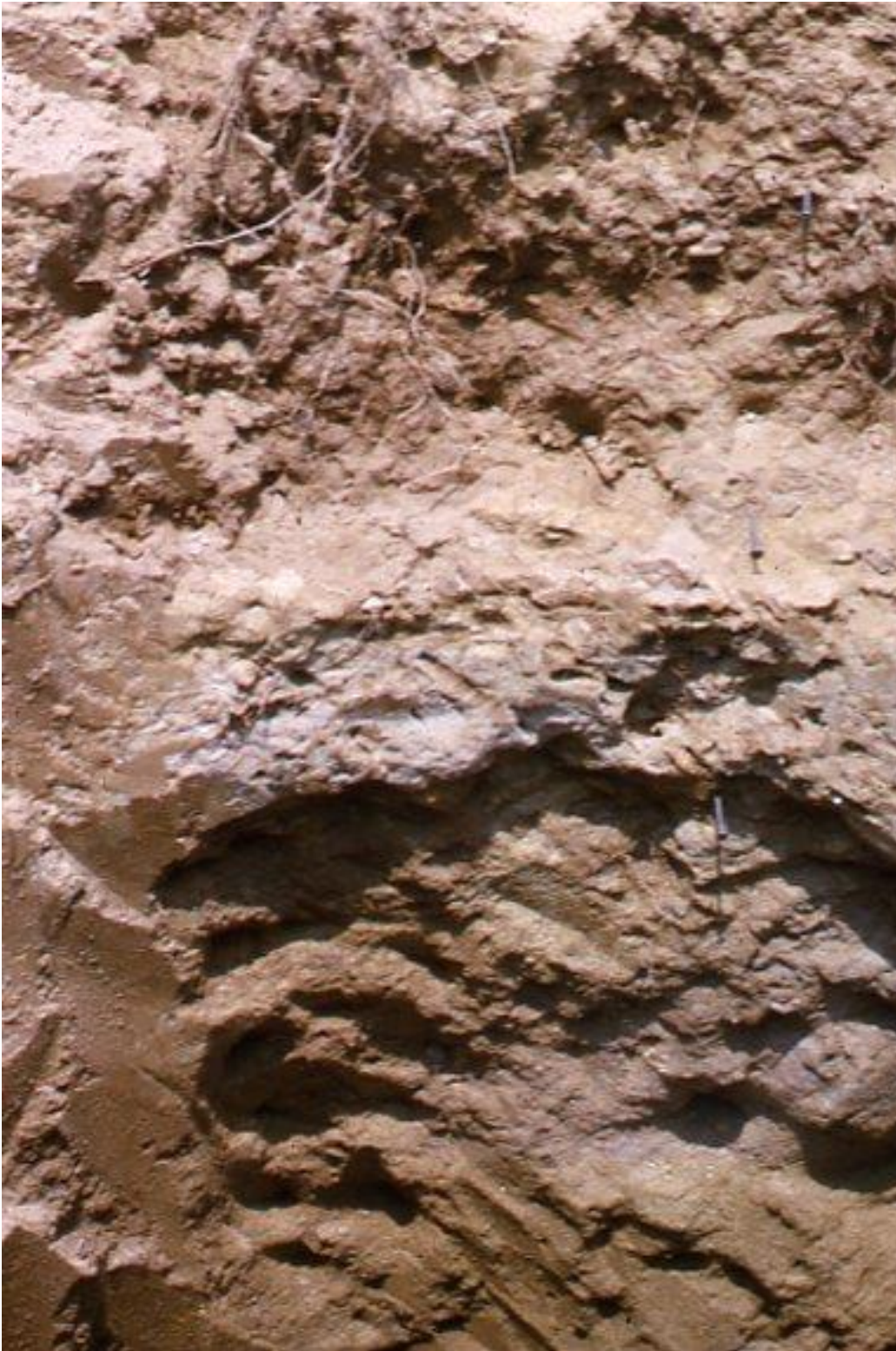
PIC 2. Silica-cemented zone with casts of shells protruding from soil pit wall in what has become designated as the Bqmj horizon are shown within the soil profile in the field. A large block of this zone (see PIC 5) was taken back to Fanning's lab/office, a picture of which is displayed in Fig. 3 and the zone in monolith is pictured in Fig. 2 of Fanning et al. (2010) paper.
