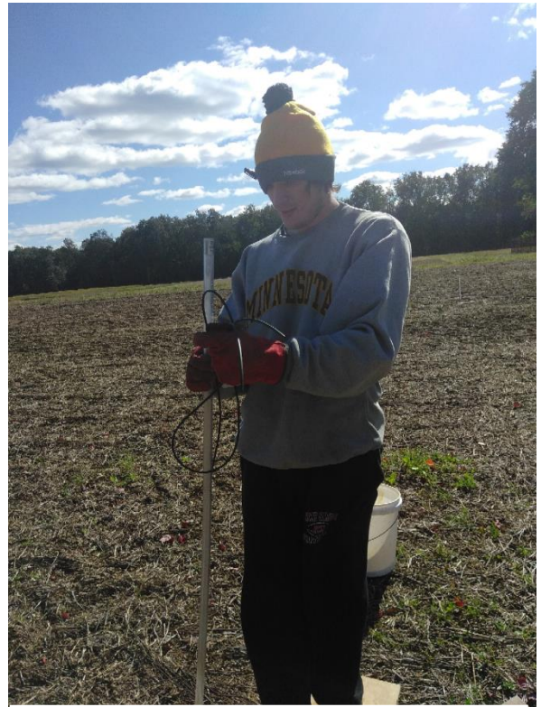
Figure 1: Ian Goralczyk, an undergraduate researcher in Dr. Ray Weil's Soil Quality Laboratory, is shown installing a suction lysimeter for collecting soil porewater samples.
