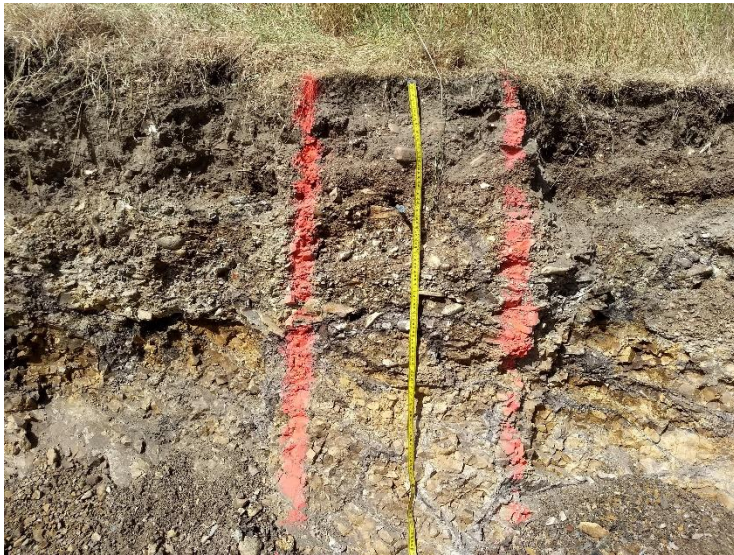
Alluvial fan deposits containing imbricated gravels over Cr horizons in a dissected landscape.
